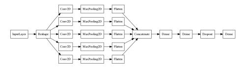
Fig. 4. The CNN structure contains five kinds of filter sizes (from 2 to 6). Each filter size contains a convolutional layer followed by a max-pooling layer. Two fully-connected layers are added after the max-pooling layers. The active function is *sigmoid* for the output layer and *Relu* for convolutional layers and fully-connected layers. A dropout layer is applied to avoid over-fitting.
